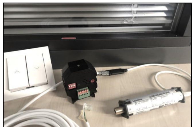
(8) Interial® I-06 Modell 1 Taster, Kabel, Controller, Motor.
